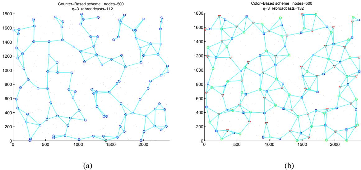
Fig. 2. Random realizations of the backbones for (a) counter-based, and (b) color-based schemes, both with threshold  $\eta = 3$ .
