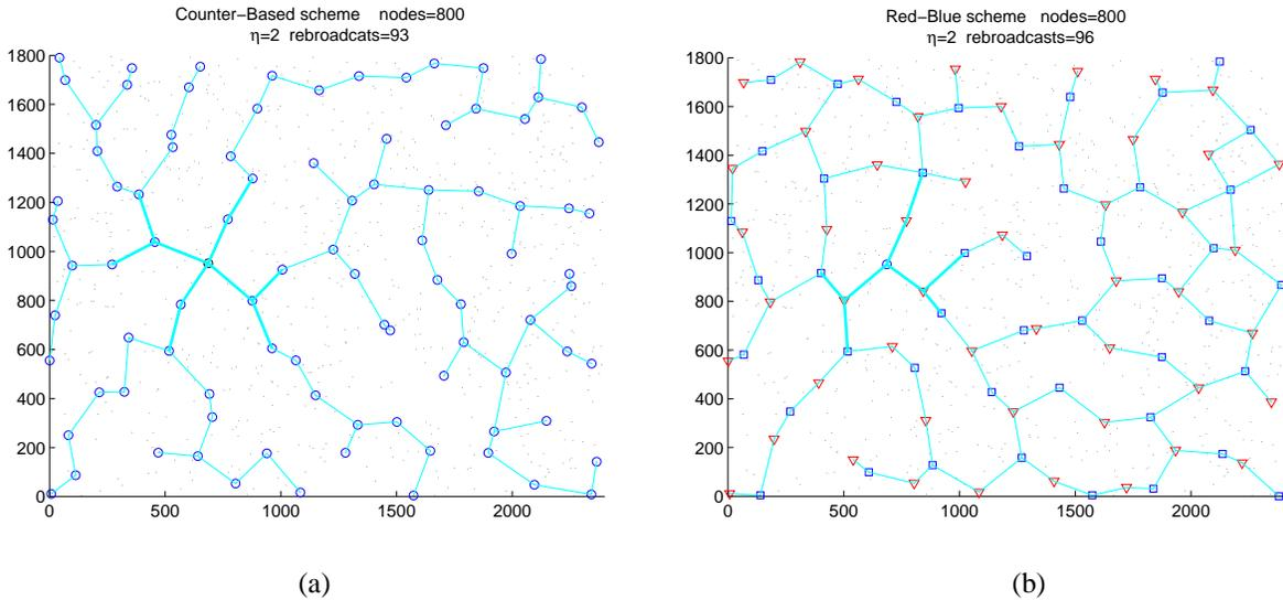
Fig. 1. Random realizations of the backbones for (a) counter-based, and (b) color-based schemes, both with threshold  $\eta = 2$ . Note the tree-structure of the counter-scheme which contrasts well with the mesh-structure of the color-scheme. While slightly larger than trees, meshes are more robust against failure.
