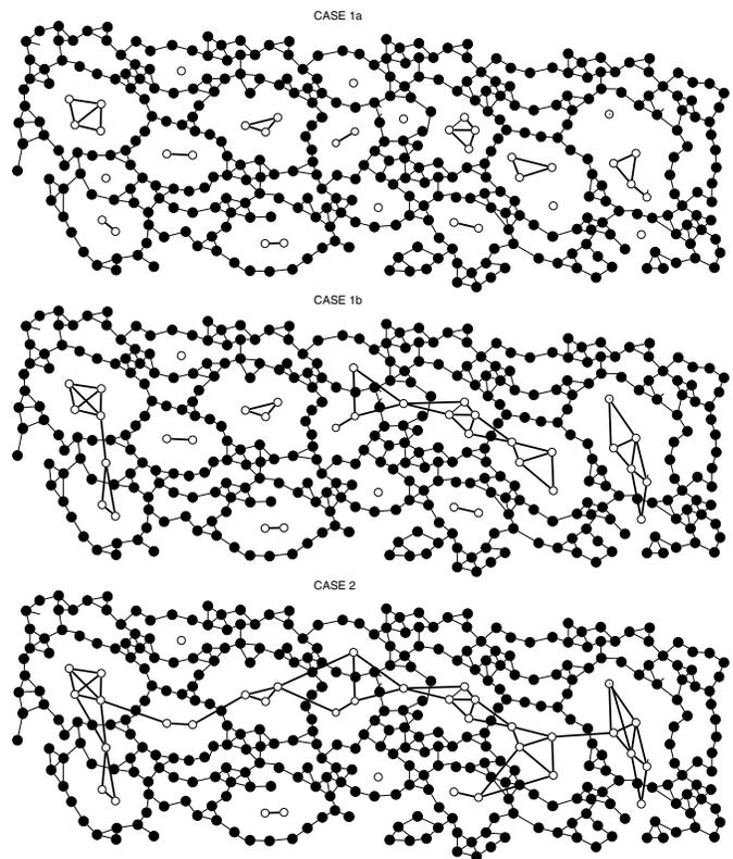
Fig. 3. The structure of the communication network. The black nodes belong to the collision-free “core”  $C_\infty(\lambda, R_F)$  while the white nodes form  $H(\lambda, R_T, R_F)$ . The connections between white and black nodes are not shown not to overload the picture.
