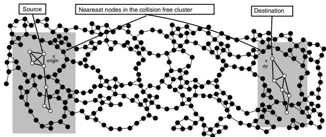
Fig. 4. Constructing a bound for latency: the black nodes form the unbounded cluster of  $\mathcal{B}_\lambda(R_F/2)$  and white nodes belong to the unbounded cluster of  $\mathcal{B}_\lambda(R_T/2)$ . The connections between black and white nodes are not shown in the picture.
