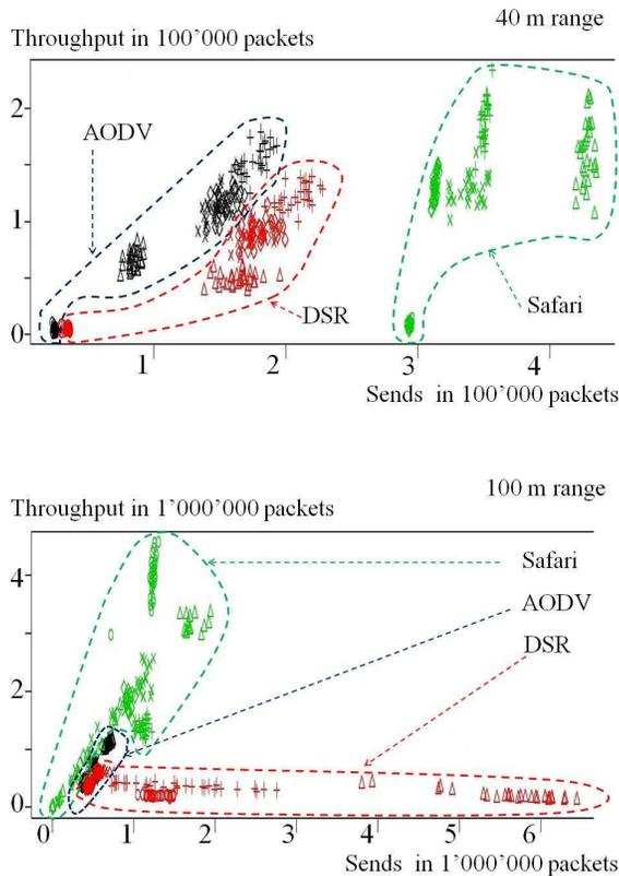
Fig. 6. Throughput by Sends for correlated sessions (random sessions see text). Range: 40m on top, 100m on bottom. Protocols: AODV black, DSR red, Safari green. Mobility models: RWP  $\circ$ , RWP(SST)  $\Delta$ , RWP(CS)  $+$ , RiceSims(SST)  $\diamond$ , RiceSims  $\times$ . Each data point represents one simulation run with the indicated protocols and settings.
